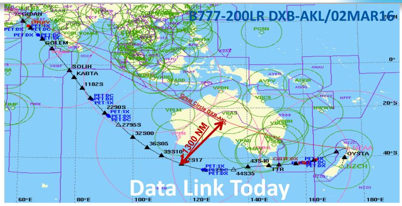
Trip Time: 15:29 / Block Time: 15:55 / Trip Fuel: 121350 / GND DIST: 8010NM / GC DIST: 7683NM
