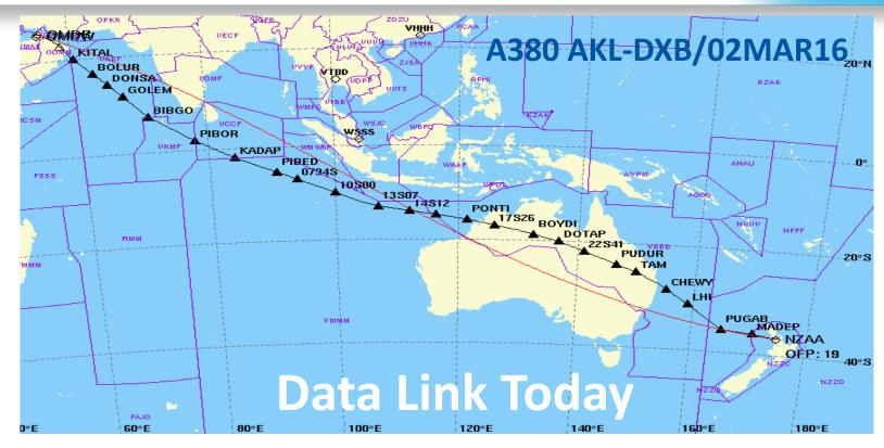
Trip Time: 16:32 / Block Time: 17:15 / Trip Fuel: 217652 / GND DIST: 8020NM / GC DIST: 7683NM
